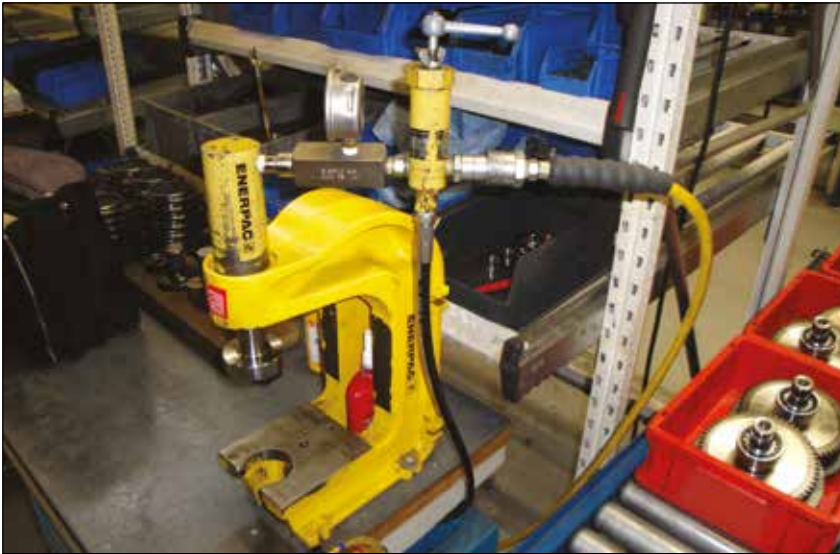
▲ RC308 cylinder mounted in A330 Arbor Press powered by a PATG-Turbo Air pump for controlled pressing of bearings for sprockets of weaving machines. The V152 Pressure Relief Valve controls the pressing force.
