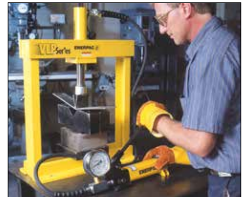
▲ VB10 V-Blocks are used in this VLP106P142 bench press to bend flat steel bar. The hydraulic pressure can be checked with the gauge.
