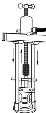
◀ Bearing Cup Puller shown with Cross Bearing Puller attachment.
