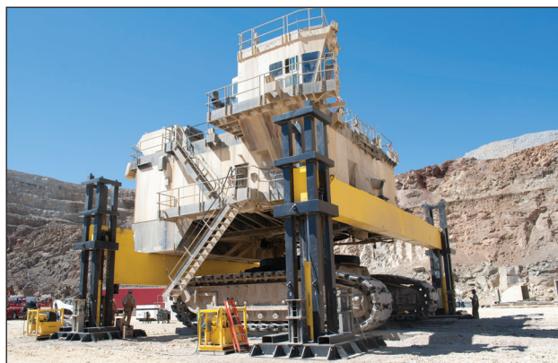
◀ A 1200-ton electric mining shovel being separated using custom 500-ton RR-Series cylinders and a pump per point synchronous lift system
