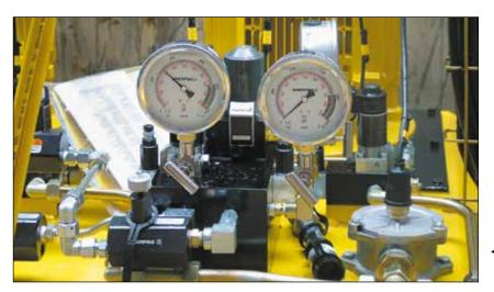
When lifting or pressing, always use a gauge. A gauge is your 'window' to the system. It lets you see what's going on.
