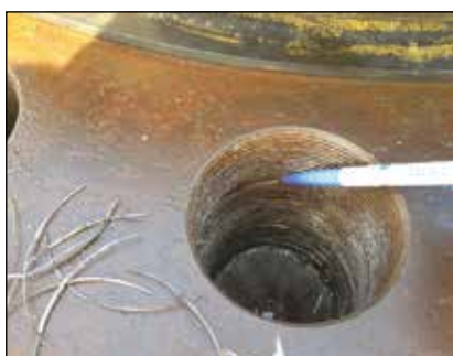
▲ A typical thread before refurbishment
