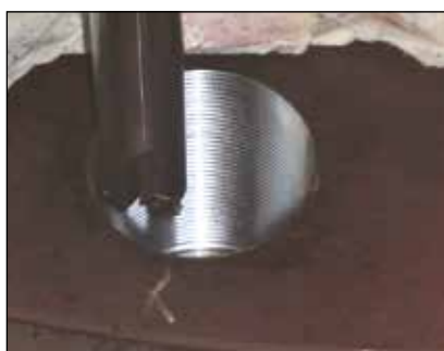
▲ New machined thread
