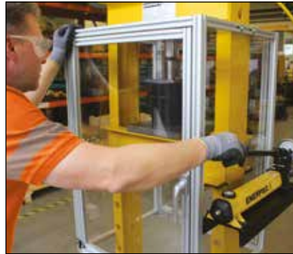
▲ Press with safety cage to ensure additional operator safety.
