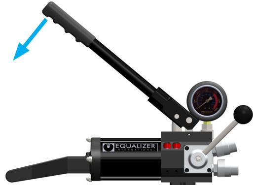
4. Steps 2 & 3 are repeated, which will pump oil into the system until the maximum pressure of 10,000 psi (700 bar) is achieved, at which point the safety release valve will open and the oil will cycle back to the reservoir.
