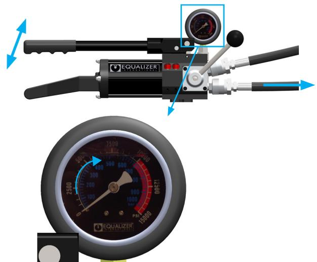
5. To depressurise the advance hose move the control lever to the retract position this will redirect the flow to the retract hose.
