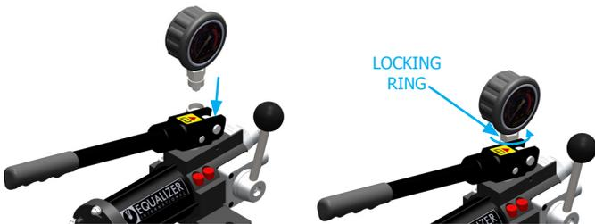
2. Ensure the hydraulic system you wish to pressurise has been bled and is free from air and leaks. Connect the pump into the system using the screw connector supplied with the pump, push the male and female connectors together fully and rotate the locking ring clockwise until fully tight.
