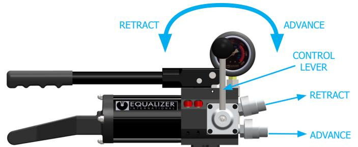
4. Pressurise the advance hose by raising and depressing the pump handle until the desired pressure is indicated on the pressure gauge N.B. max. pressure 10,000 psi (700 bar)
