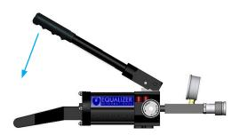
Steps 2 & 3 are repeated, which will pump oil into the system until the maximum pressure of 700 bar (10 000 psi) is achieved, at which point the safety release valve will open and the oil will cycle back to the reservoir
