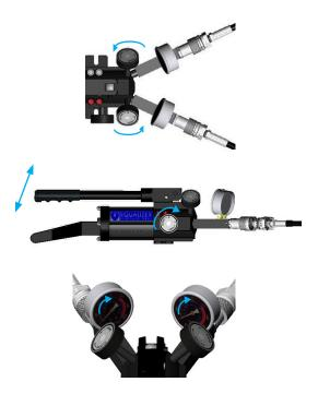
**b.** If control valve 1 is open and control valve 2 is closed with the release valve screwed fully home, when the pump handle is raised and lowered only the system connected to control valve 1 will be pressurised (max. 700 bar (10 000 psi)).
