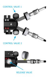
**a.** If control valves 1 and 2 are set to the fully open position and the release valve is screwed fully home, when the pump handle is raised and lowered both hydraulic systems will be pressurised to an equal pressure (max. 700 bar (10 000 psi)).
