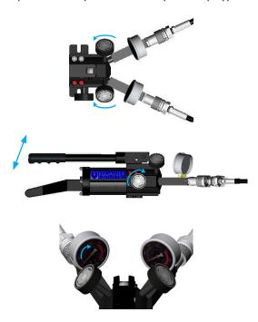
**c.** If control valve 2 is open and control valve 1 is closed with the release valve screwed fully home, when the pump handle is raised and lowered only the system connected to control valve 2 will be pressurised (max. 700 bar (10 000 psi)).
