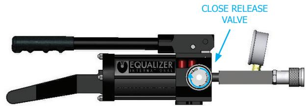
4. Pressurise the system by raising and depressing the pump handle until the desired pressure is indicated on the pressure gauge. N.B. max. pressure 700 bar (10 000 psi).
