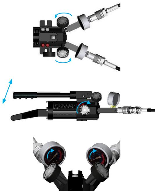
**c.** If control valve 2 is open and control valve 1 is closed with the release valve screwed fully, when the pump handle is raised and lowered only the system connected to control valve 2 will be pressurised (max. 700 bar (10 000 psi)).
