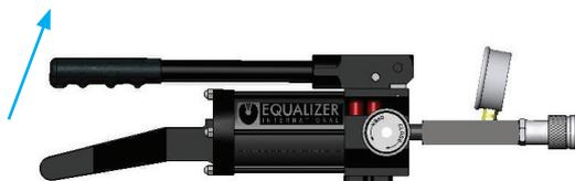
The pump handle is depressed, which pumps the oil from the chamber through the outlet port and into the system to which the pump is connected
