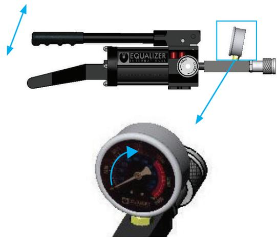
5. To depressurise the system, gently open the release valve by rotating the release knob anti-clockwise
