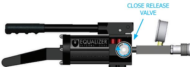
The pump handle is raised, which creates a vacuum in the piston chamber which sucks oil from the reservoir into the chamber
