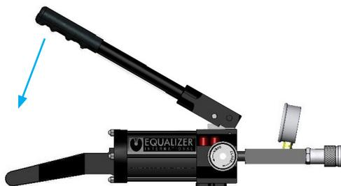
Steps 2 & 3 are repeated, which will pump oil into the system until the maximum pressure of 700 bar (10 000 psi) is achieved, at which point the safety release valve will open and the oil will cycle back to the reservoir
