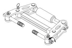
Pull the Collet Spring Plunger Ring to release and remove the collet head assembly.
