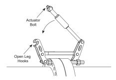
Tighten the actuator bolt until the lugs on the actuator union engage in the hooks on the open legs.
