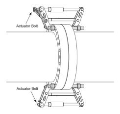
When the torque wrench clicks, stop and increase the torque wrench setting by 10 N·m [6.5 ft·lb]. Continue to tension both tools evenly until the flange spreads or the torque wrench clicks.
