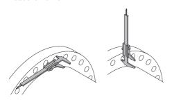
To read the measurement from the vernier calliper, scan along the desired scale from left to right. In this example, the major figure is 60 mm, this is added to the minor figure of 8 mm (indicated by where the vernier scale aligns with the main scale), giving a total measurement of 68 mm.
