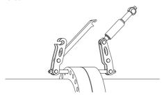
Both drive nuts are tightened, locking the tool into the flange bolt-holes.
