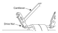
The cantilever followed by the actuator are swung and locked into position.
