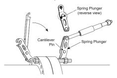
**A WARNING** Operating the tool without the cantilever fully locked into position may result in personnel injury and damage to the tool.
