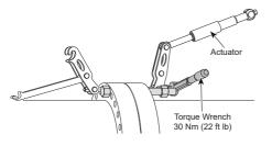
Rotate the cantilever into position hooking it over the cantilever pin in the actuator half of the tool.
