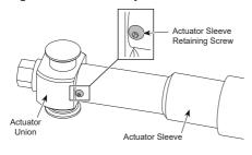
Pull the actuator sleeve back - this will expose the actuator union retaining circlip. Expand the circlip with circlip pliers and slide it up the actuator bolt by about 50 mm [2"].
