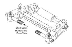
The SG11TM Short Collet Kit comprises a pair of Short Collet Holders and Drive Cones, but is not supplied with Collets or Springs.
