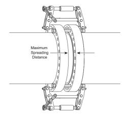
**A WARNING** The Secure Grip mechanical tools are fitted with an internal mechanical stop which limits the travel. Forcing the tool to travel further will result in tool failure.
