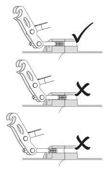
If a spacer, blind or valve is installed between the flanges, care should be taken to ensure that the Collet or Collet Holder do not extend beyond the flange bolt hole.
