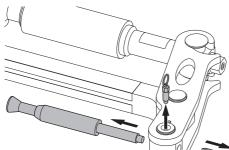
Remove the Drive Cone and Collet from the Collet Holder. Replace the Collet with the applicable size for the flange joint as selected in Section 5.2.
