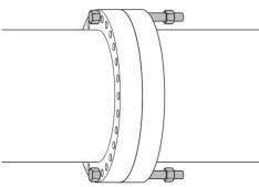
The collets are suited to the sizes of the bolt-holes and should be selected prior to commencing work by following the instructions in this section.
