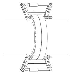
**ACAUTION** If more than two tools are being used they should be attached at an equal spacing around the flange joint.
