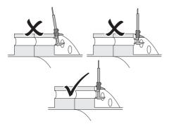
To confirm that the bolt-hole is round, take two separate measurements with the vernier calliper turned through 90° between measurements.
