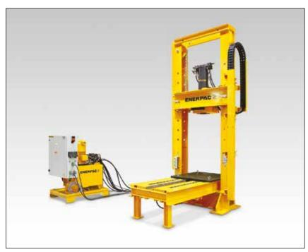
▲ For offshore application high capacity spring loaded cylinders need to be assembled and tested. A special 100 ton roll frame press, with long stroke cylinder has been constructed. All movements are operated and monitored through a PLC controlled pendant.
