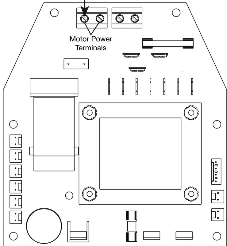
*Figure 9, Connection to Power Board - 115V and 230V Fans (LCD equipped pumps only)*
