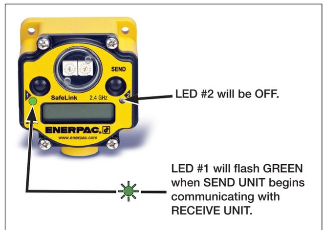
Figure 12, Communication In Progress - SLS Send Unit
