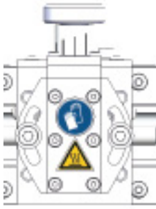
Figure 1: Tool holder showing safety labels
