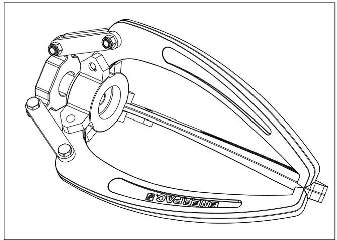
Figure 5, Long jaws installed and straps attached.
