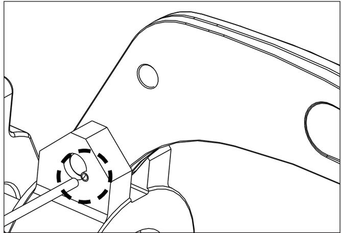
Figure 4, Restoring peened area after installing pin.
