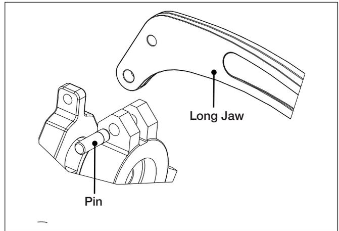
Figure 3, Long jaw installation.
