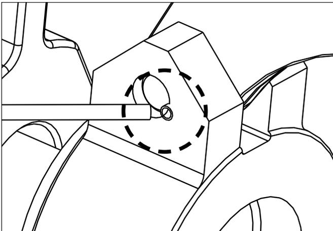
Figure 2, Removing peened area to allow pin removal.
