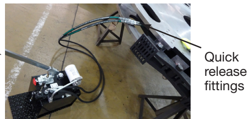
Figure 14: Hydraulic base pump connection.
