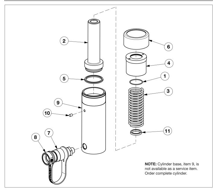
**A WARNING** STOP RINGS ON RCH MODELS ARE SPRING LOADED! If not contained during disassembly, spring and stop ring could cause personal injury.
