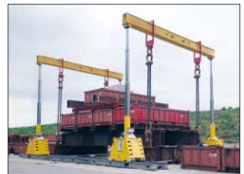
SL400 Gantry during load testing. ►
