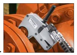
Slim enough to fit and tough enough to last. This UltraSlim wrench is the perfect controlled bolting solution for this oil and gas flange.
