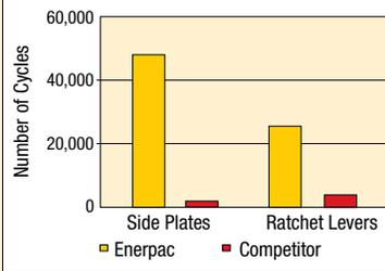
\*Average test results, whereby three Enerpac 1<sup>3</sup>/<sub>16</sub>" UltraSlim cassettes and three competitor 1<sup>3</sup>/<sub>16</sub>" cassettes were tested at 4000 ft-lbs for 50,000 cycles. The Enerpac side plates never broke for the full duration of the test.
