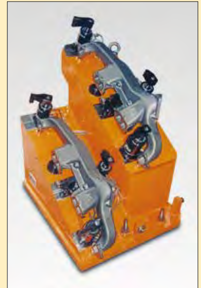
■ MPTL-100 and MPTR-100 Collet-Lok® Swing Clamps are used to securely clamp these exhaust manifolds.
