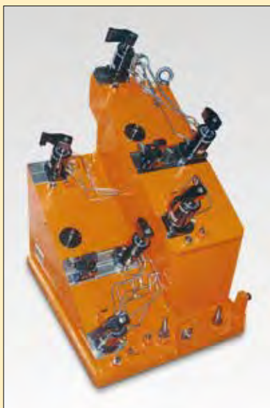
■ Fixture for machining exhaust manifolds.
