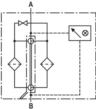
Duplex filter without by-pass valve and with mechanical indicator as well as pressure equalization line
